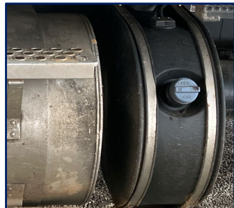
Closeup of DEF system
