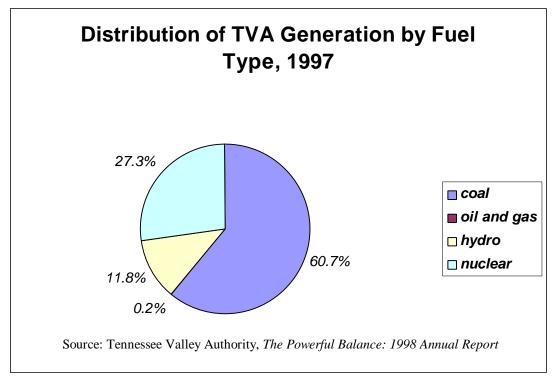
TVA has a slightly lower percentage of coal-fired generation and considerably less gas-powered generation than the rest of the country, and it has more hydro and nuclear power. The larger
