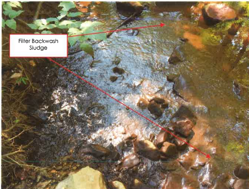
Photograph 4 – Filter Backwash Sludge in Stream
